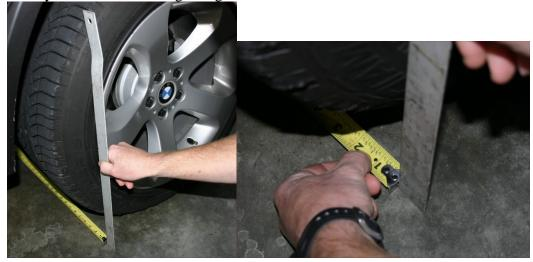
3. Go to the other side of the vehicle. Hold straight edge in exactly the same position (where tire and rim meet), and slide the straight edge down against the tape measure. Read where the two touch, on the shorter side of the tape. In this example, it is 67 3/4"
