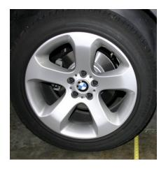
2. Once tape is under vehicle, hold straight edge firmly against the tire and pull tape firmly against it. The tape should sit firmly on the ground, and should hold its' position when you remove the straight edge.
