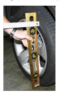
If you don't have a camber gauge, simply use a level (3' is good) and a tape measure or ruler. Again, move level away from bulge, halfway from center-of-rim to rim-edge works fine on most cars.
