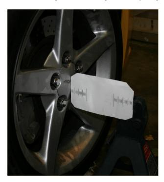
2 Hold laser level against rear wheel. Depending on how wide your body work is, you can either hold it against the rim seat, the rim lip, or the tire itself. You MUST PUT IT IN EXACTLY THE SAME PLACE WHEN YOU DO THE OTHER SIDE OF THE CAR.
