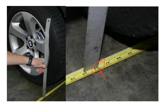
4. Repeat steps 1-3 on the back of the same 2 wheels. Measure that distance and simply calculate the difference. For instance, if the front of the tire measure 67 <sup>3</sup>/<sub>4</sub>" and the rear measure 68 <sup>1</sup>/<sub>4</sub>", then your tires would be toed-in <sup>1</sup>/<sub>2</sub>" TOTAL.
