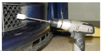
11. Insert the eye hook through the grill and screw it into place. Use a drop of lock tight if you plan to leave the hook in place for extended periods.
