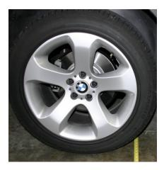
2. Once tape is under vehicle, hold straight edge firmly against the tire and pull tape firmly against it. The tape should sit firmly on the ground, and should hold its' position when you remove the straight edge.
