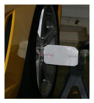
4. Repeat on other side of car. Difference between the two measurements is your thrust runout. If you can get it within 1/8" (less than 0.1 deg), your are in great shape. Remember, you aren't measuring track width or anything, just need a RELATIVE differential between your front and rear offsets. You MUST place your tools and make your measurements exactly the same on both sides.
