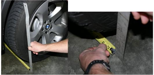
2. Go to the other side of the vehicle. Hold straight edge in exactly the same position (where tire and rim meet), and slide the straight edge down against the tape measure. Read where the two touch, on the shorter side of the tape. In this example, it is 67.34"
