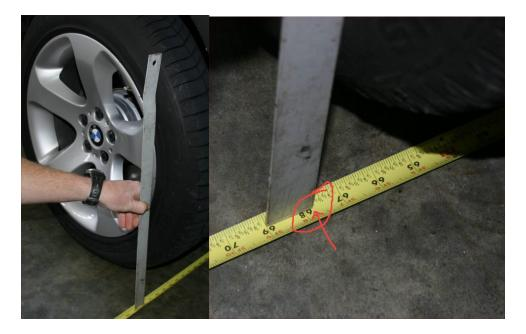
Repeat steps 1-3 on the back of the same 2 wheels. Measure that distance and simply calculate the difference. For instance, if the front of the tire measure 67 <sup>3</sup>/<sub>4</sub>" and the rear measure 68 <sup>1</sup>/<sub>4</sub>", then your tires would be toed-in <sup>1</sup>/<sub>2</sub>" TOTAL.
