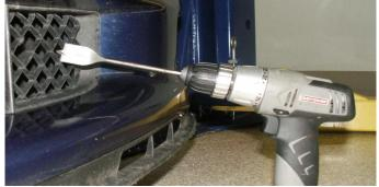
9. Insert the eye hook through the grill and screw it into place. Use a drop of lock tight if you plan to leave the hook in place for extended periods.
