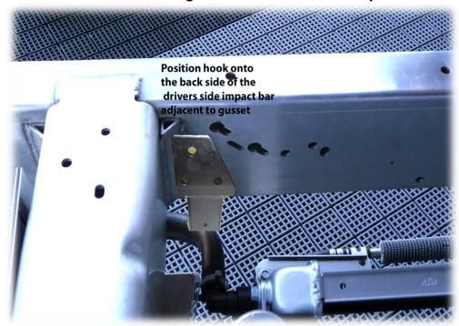
2. Remove the paper on the side of the double stick tape (tape provided) and press bracket into position to drill the 3/8" pilot holes. Using the air wrench with the 3/8" bit, drill the top pilot hole first and then place a 3/8" bolt in the hole to ensure that the bracket stays properly positioned for drilling the other holes. Drill the other 3/8" pilot holes. The speed of the air wrench is slow which helps control the drilling process. Frequently oil the bit to keep it sharp.
