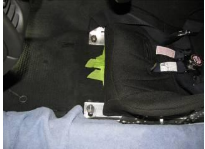
Seat rails fastened to Stud Extenders
