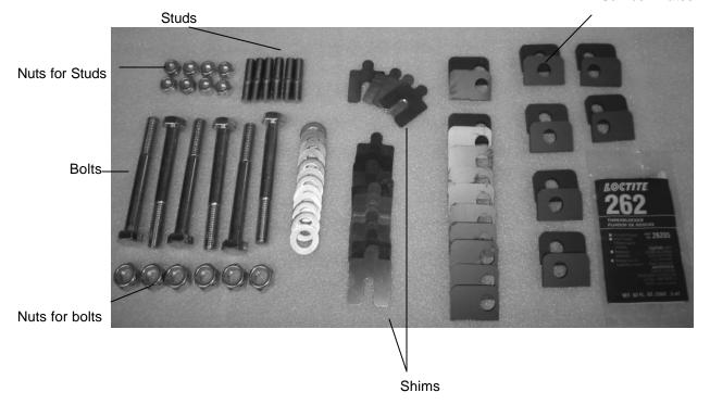
The purpose of this kit is to simplify the alignment process and correct the factory shortcomings. The orange camber plates have different hole placement and are identified by the notches on the bottom.
