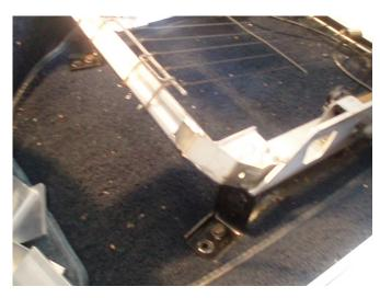
Align the front two legs so that the back hole aligns with the existing mounting location. This is why the legs are at an angle. You will have to be sure that you keep the frame square to the car. Once you get this done, remove the frame and put thread lock on the front leg bolts and tighten it down. You are now done with your frame modifications.
