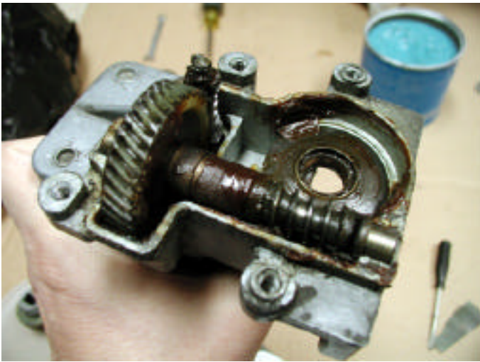
Note that the black curved washer faces curve up toward the removed pot metal gear. Next goes the silver metal washer, then the pot metal gear, then the nylon gear. Be sure to clean the old grease off of everything before reassembly.
