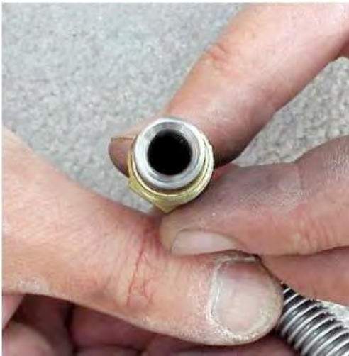
Final flared tube end after clean-up. Note spiral wrap armor installed over the tube section.
