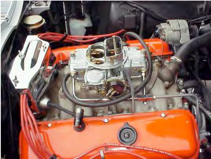
1-piece steel fuel line installed on a Holley with in-carb filters
