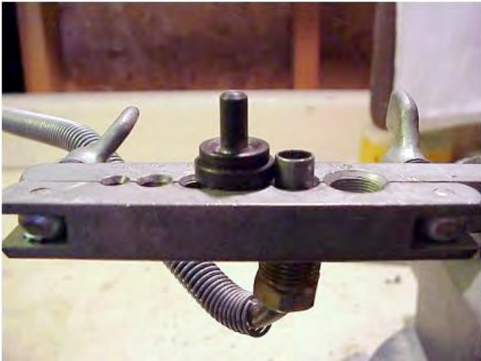
This is how much tube you must have sticking out of the flaring tool after the cut. Anything less, and you won't be able to complete the flare. Any more, and the tube will stick too far out of your fuel pump.
