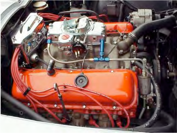
Completed in-line filter line with "O"-Ring fittings at filter and AN fittings at Demon carb.
