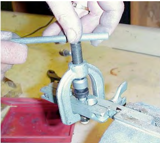
The tube end being “crushed” by the double-flare spacer in the first step of the operation.
