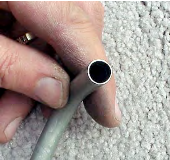
Here is the finished, properly prepped tube end. No burrs, ridges, or defects of any kind.
