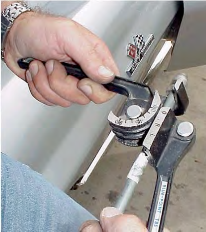
Bending up the upper section of the in-line filter line.
