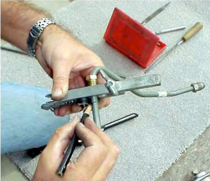
Marking the tube for cut length with the flaring tool in place.
