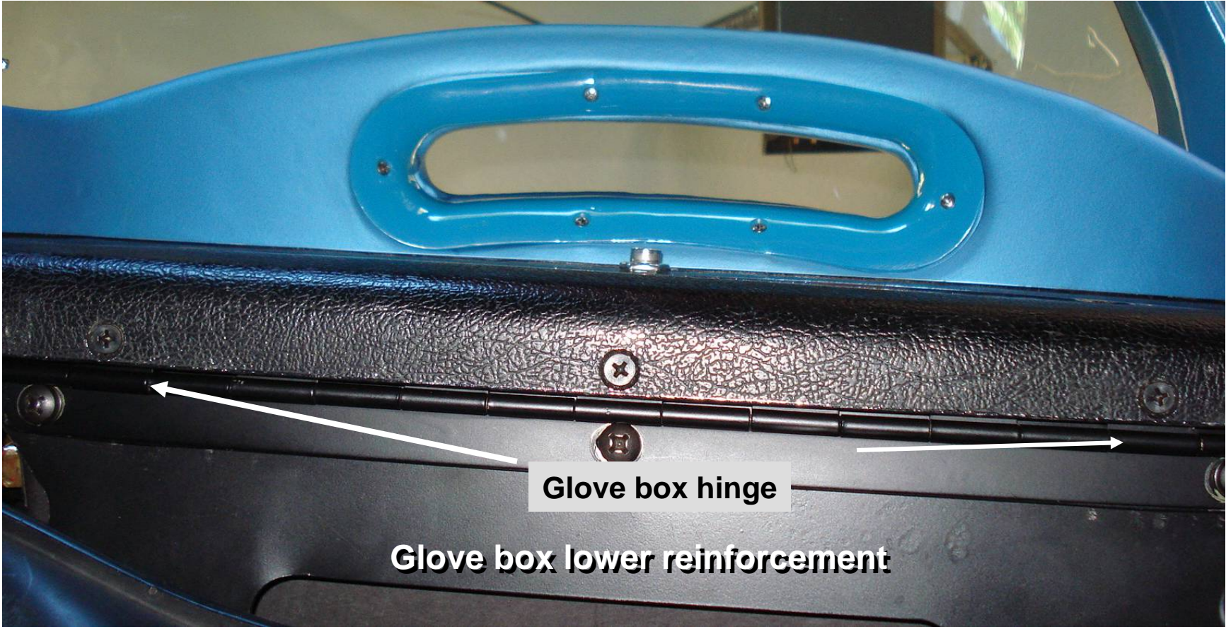
Hinge and reinforcement viewed from below
