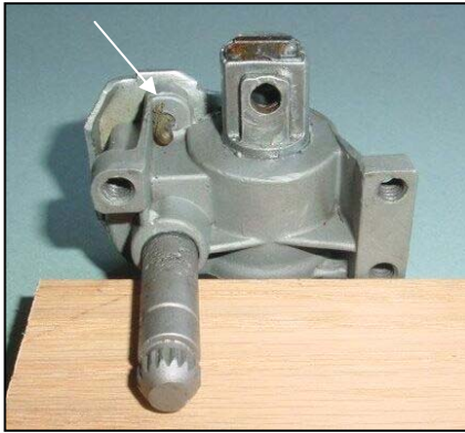
“Front” view of vent-window regulator
