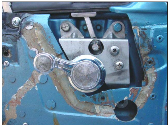
Vent-window regulator installed in door
