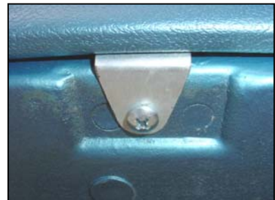
Installed panel clip
