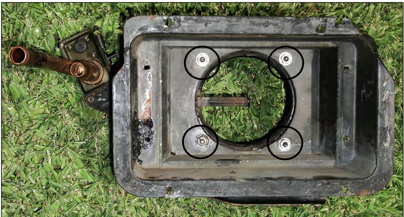
Heater box with core removed. The four nuts and washers retain the studs on the blower housing. The bracket in the center holds the capillary tube.
