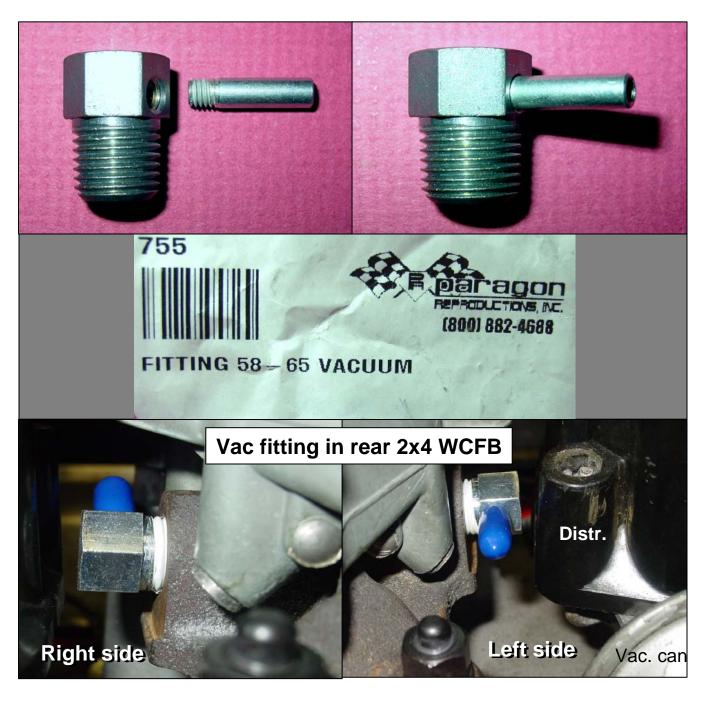
This is the vacuum fitting that you can get from Paragon. The little side arm has 10x32 threads (don't ask me how I know). My 60 is currently set up with a vacuum advance distributor (incorrect but working nicely) and this is where I attached the vacuum line. Note the position of the vac can in the lower right photo. The distributor and plug wires have been reindexed to allow the vacuum advance distributor to clear the manifold.
