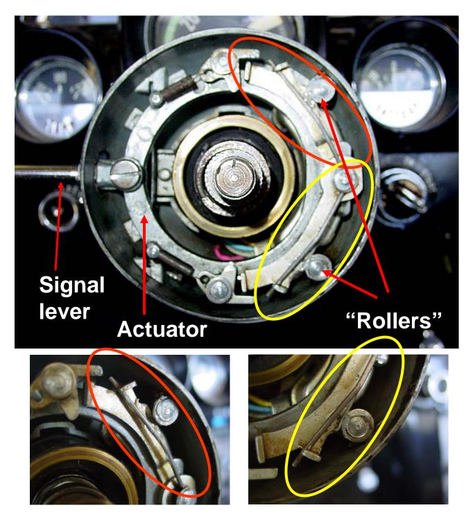
Turn signal mechanism rocks back and forth on the rollers shown above.
