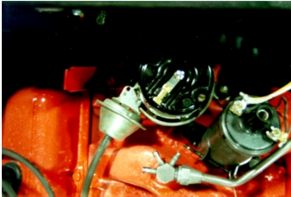
Figure 1: Distributor & Rotor Correctly Installed at #1 Firing Position
