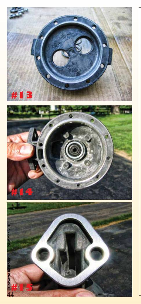
link while pushing down on the diaphragm/ stem assembly. This will disengage the hook in the end of the link from the slot in the upper section of the diaphragm stem. If you have trouble with this after a few attempts, then put it down for a while. Go inside the house and kick the dog. Have a coupla brewskis and return to trying to drive the diaphragm stem seal out of the housing.
