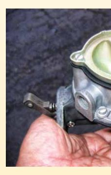
Insert the original retainer pin and washer in the same orientation as it was when you removed it. Place the X marked end onto an anvil or vise, and, using a small cold chisel and light hammer, gently deform the pin by re-spreading the same grooves that you squeezed together upon disassembly (fig. 21). Insert small return spring between rocker arm and upper casting (fig. 22).
