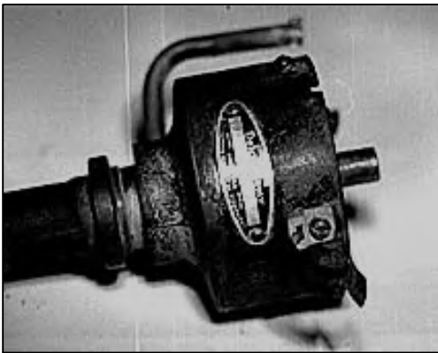
Photo depicts the Delco-Remy Part number plate on distributor #1110847, which is located on the external face of the distributor bowl by rivets. Although not easy to see, the date code reads as 4-M-17 (1954, DECEMBER, 17TH DAY).
