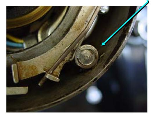
Close-up of rollers shown in previous photo. These were a bit gunked up on the car when I got it. A little PB Blaster or Kroil and they roll very well.
