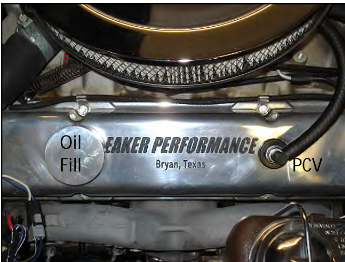
Connection from vacuum fitting at rear of carb to left valve cover
