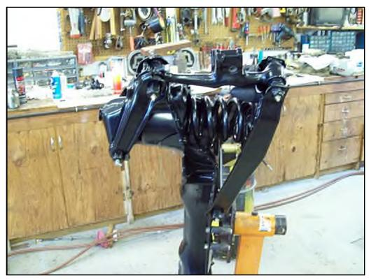
The final part of assembly is installing the spindles onto the spindle supports with new kingpins and bushings. I explained earlier about honing the bores for a "slip fit" of the bushings. Each bushing has a hole for grease to enter the bushing. **This hole is positioned in the spindle bores opposite of the hole for the grease fitting.** When bushings get greased, the grease is supposed to go all around the bushing and then into the inside to lube the kingpin.
