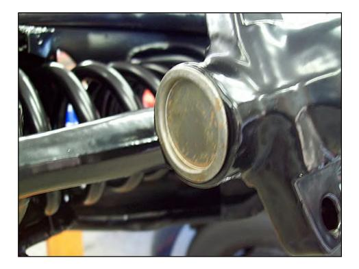
If all the grease fittings have not been screwed in place, do this now and thoroughly grease everything. After the assembled frontend is installed in the car and the weight of the car is on the suspension, bounce the car a few times and go back and grease everything.
