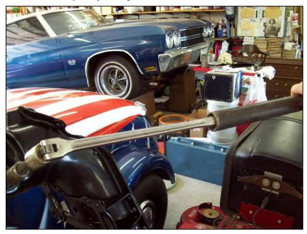
Once the shafts are installed most of the way, start measuring each end to assure they have an equal length of threads protruding from each side. **Again, critically important!**
