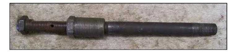
As mentioned above, installing the new upper-inner shafts is a VERY tight fit since they are oversize. **Install them dry, do not use any lubricant.** These shafts need to fit so tight that there will not be any possible chance of them turning in the cross member bushings.
