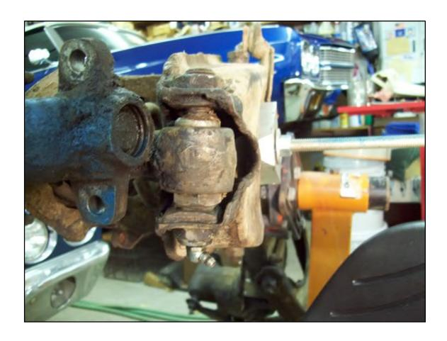
Prior to separating the spindle support from the lower A-frame, it may be desirable to separate the spindle from the spindle support. It really doesn't matter if the spindle/supports are separated at this time, or after the support is removed from the A-frames and then separated on the workbench, it's a toss up.
