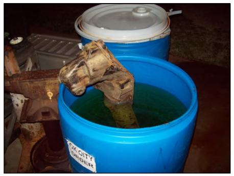
After removing the parts from the acid bath, they are THOROUGHLY rinsed off with a power washer (BE SURE to rinse very well inside of the cross member) using VERY hot water (my hot water heater is turned up to the max). After the thorough rinsing, all parts are finally blasted to get them to bare metal.
