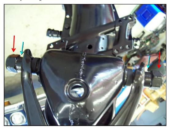
ALL grease fittings for the front end are straight, EXCEPT the REAR, upper A-frame grease fitting. It is either a 45-degree or 90-degree fitting (I've observed both styles over the years). Install the upper, rear fitting so that it points downward and slightly outward when the A-frame is in a normal loaded position.
