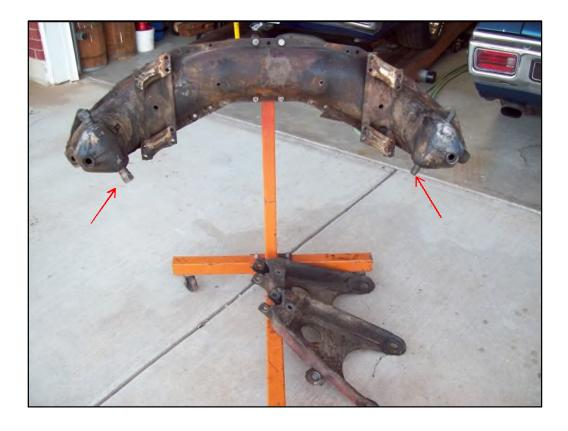
Examine the threads on each end of the shafts. If they are worn like this (below), then the threads inside bushings will also be worn and the **shaft/bushings need to be replaced**.
