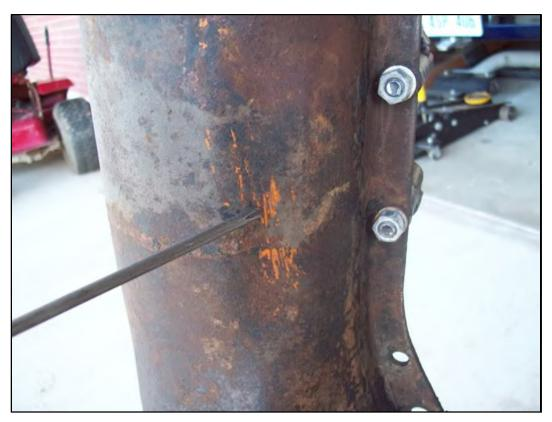
Once the cross member is completely disassembled, all that remains are the UPPER-INNER cross shafts, which are VERY TIGHTLY THREADED into the cross member.
