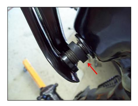
Coat the threads of the shaft with grease, then start each bushing evenly over the threaded shaft until the ends of the bushings contact the A-frame, making sure the A-frame is centered. **Where the bushing screws into the A-frame Blue arrows)**, **it needs to be dry, not lubed.** Then screw each bushing, a little at a time, all the way into the A-frame, continually checking that the A-frame remains centered.
