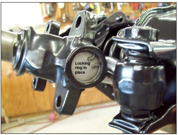
MOST kingpin/bushing kits contain two thin caps. **This thin cap ONLY goes on the top of the spindle bore.** It is necessary to gently tap it in place (they do not fit very tightly) and be careful not to deform it or it will never stay in place!
