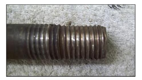
There are essentially two ways to remove these shafts. Either with a BIG pipe wrench, which will permanently damage the threads on one end, or, using the tool shown in the manual (Upper Control Arm haft Remover and Replacer - J-2958).
