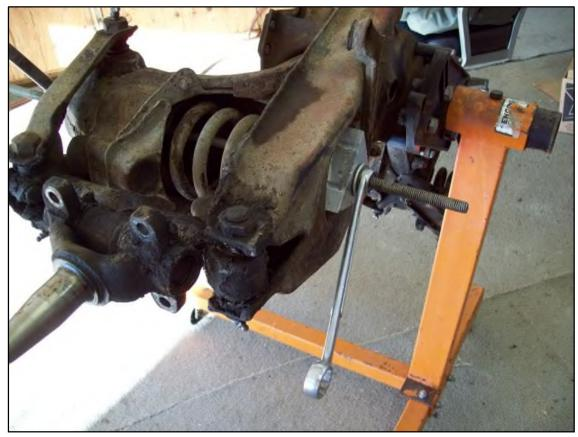
I lock two nuts together on one end of the rod which allows holding the rod securely with a wrench. Alternatively, if desired, a single nut could be welded to one end of the rod.
