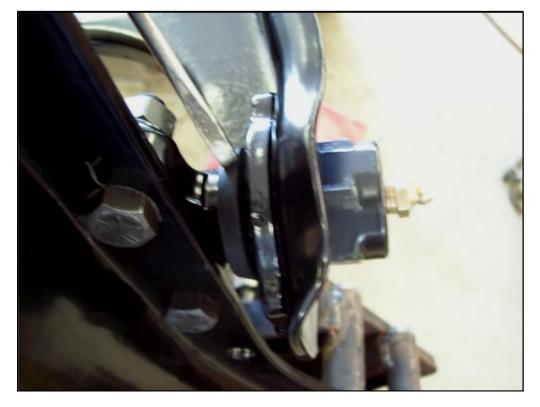
After the upper and lower A-frames are installed on their shafts, install grease fittings, shoot some grease into the bushings and work the A-frames up and down and shoot in some more grease. Now is also a good time to install the rubber bumper in the lower A-frame if not already installed.
