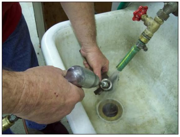
After everything is disassembled, cleaned, acid dipped, blasted and any repairs have been completed, the parts (per individual preference) are now ready for painting, powder coating or whatever finish you choose. These parts were powder coated semi-gloss black. **Some areas need to be covered with tape such as spindle ends, threaded areas, etc.** Most powder coating businesses will do this as directed.
