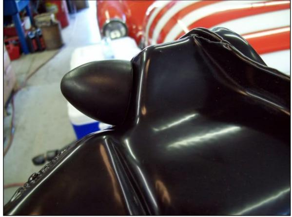
At each joint, there is some kind of rubber seal which goes over the shaft threads to keep "crud" out of the shaft/bushing seals. The rebuild kits may or may not come with good seals; Paragon sells a kit containing all the seals needed for a complete front end.
