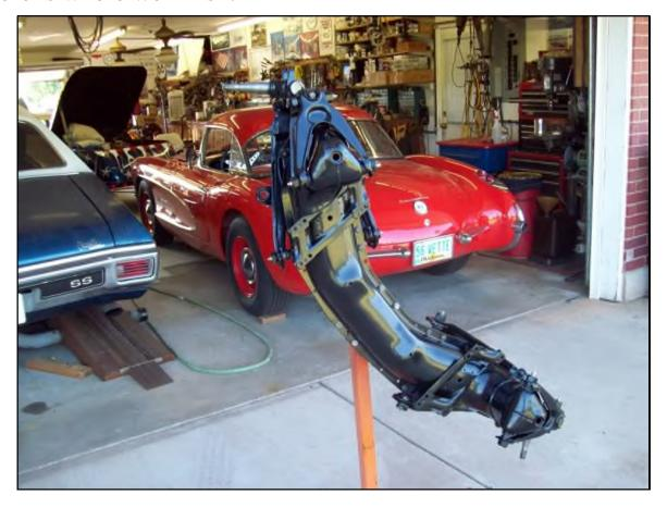
The frontend rebuild in the following pictures is from a 57 Corvette which appeared to have never been rebuilt. Also, it is very representative of all 49-54 Chevy passenger car and 53-62 Corvettes.
