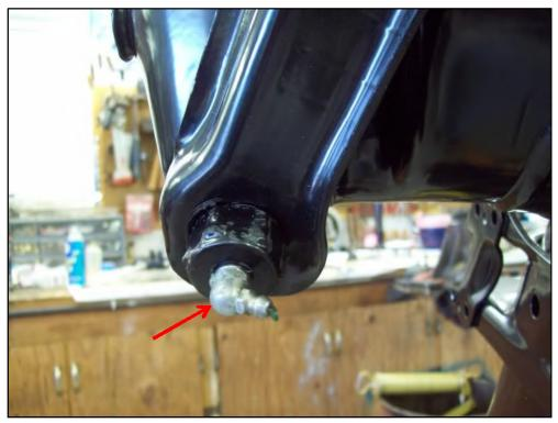
Installing the lower A-frame can be done by either attaching the cross shaft to the cross member, or, by installing the cross shaft to the lower A-frame and then bolting the shaft to the cross member. I prefer to install the shaft to the cross member first-----WITH NEW GRADE 8 BOLTS!
