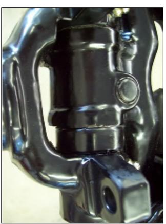
Once the spindle, kingpin, bushings, shims and bearing are assembled to the spindle support and you're satisfied the spindle rotates with the correct amount of stiffness (this is a subjective "feel" thing gained from experience), it's time to install the plugs and snap rings in each end of the bores.
