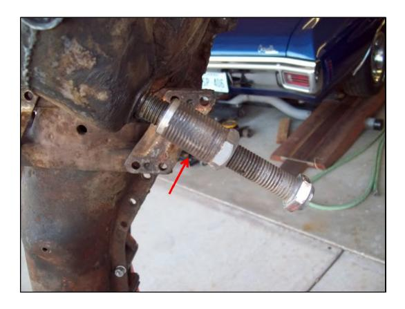
It's not uncommon to discover that the upper-inner shaft is "sloppy loose" in the welded-in bushings (arrow below) due to poor past maintenance (i.e., failure to keep the suspension joints greased).
