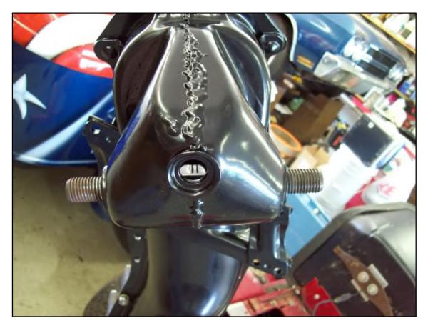
Now is a good time to do little things, such as installing the new rubber bumpers for the upper A-frames. Spray a little silicone on the end, insert it into the hole at an angle and with a pushing, twisting motion, twist it into the hole.
