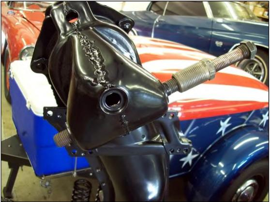
A breaker bar and "cheater" may be required to get the shafts installed.
