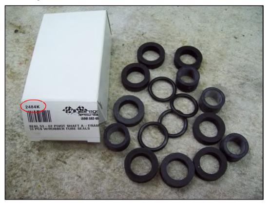
Prior to installing the upper A-frame, slide a seal over each end of the shaft threads, slip one end of the A-frame over the shaft then slip the other end of the A-frame over the shaft. With the seals in place, it may take some concentrated tugging on the other end of the A-frame to get it pulled over the shaft.
