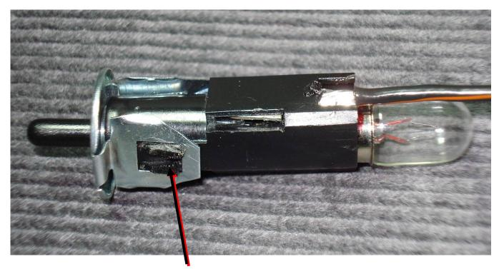
To disassemble the switch trim the melte Postic plastic from this area and gently pry metal side tabs up over remaining plastic. Preserve as much as you can.
