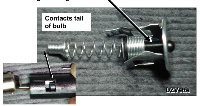
When Glove-box door is open the push button releases the spring which moves forward to make contact with the grounded metal housing closing the circuit to light the lamp.
