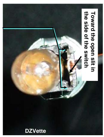
Connector slips in here. Open side of the "hook can be seen in the slit at the upper right of the switch housing.
