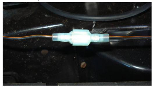
Consider adding a quick-connect in the Blk/Or wire to the glove-box lamp. It will eliminate having to wrestle that connector out of the lamp housing which can be problematic. Makes Glove Box removal easier in the future!
