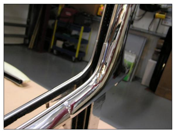
Here are some photos with the glass used for a test fit. The front frame of this window glides easily past the corners and fits well. Because I removed that thick area at each fuzzy corner there is no resistance to bind up the frame. At the rear end of the fuzzies, the frame may bind slightly.
