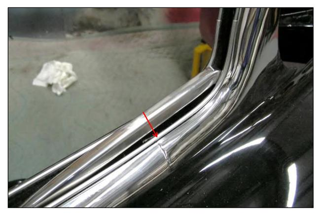
After the grinding for excess chrome removal, all 4 trim pieces now fit properly. You can see how much material needed to be removed.
