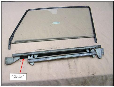
The rubber gutter has a channel which grips the glass. It may be stuck on there so you can use a soapy water solution to help free it up.
