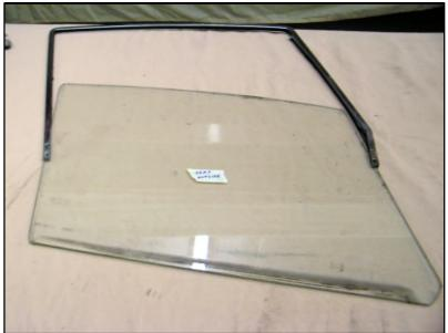
Separate the old seal from the frame. Clean the glass along the edges using a solvent to help remove the old seal residue.
