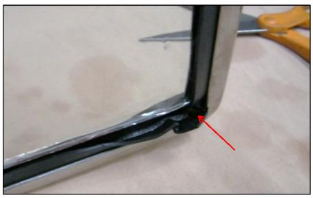
Lay the top edge of the frame, face down, on a padded solid surface. Push down evenly to seat the glass as far as possible.
