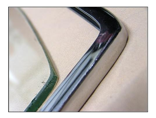
Clean the sash and install the new gutter seal. Note the orientation. When installed, the gutter is to the outside of the door. Note the original markings from the manufacturer of the sash and the oval symbol "Elkhart Indiana".
