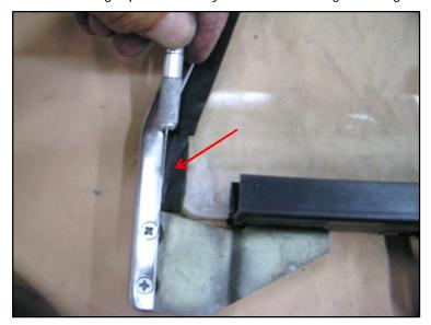
Trim the sash gutter rubber seal at the front end as the original was (right of photo below). This prevents clearance issues when installing the assembly back in the door.
