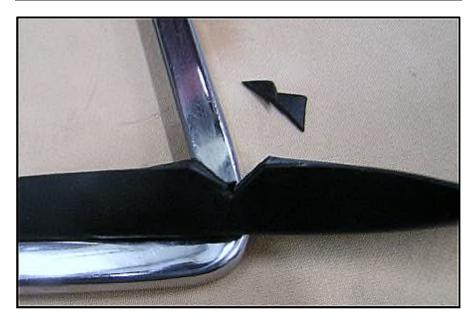
Apply more solution to the inside of the sealing tape. Start the glass into the frame. You may have to spread the frame a bit to get it past the bent corner of the glass. Get it down to the channel and carefully push down against the frame. Make sure the sealing tape in the corners is spread open to receive the corners of the glass.
