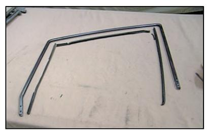
Now that the frame is released from the glass it can be cleaned and buffed to a brilliant shine. Also wire brush the inside of the frame to remove any old seal material or dirt.
