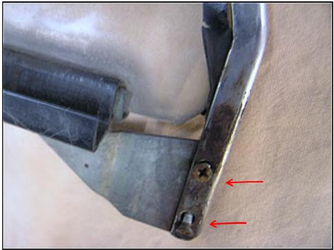
Using an awl or small screwdriver in the holes of the frame, carefully pry the sash from the glass. Do not pry on the edge of the glass.
