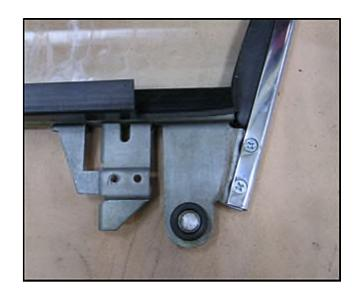
Using a sharp pointed blade, trim the sealing tape all the way around at the edge of the glass/frame on both sides.
