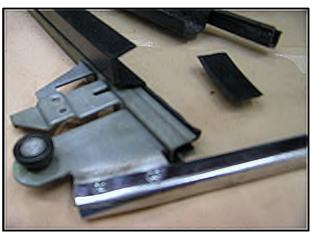
Clean or refinish the lower track guide and install for later. Note this must be removed for installation of the glass assembly into the door, as the window is installed first and the track is slid onto the 2 window regulator rollers then attached with the 4 screws to the sash.
