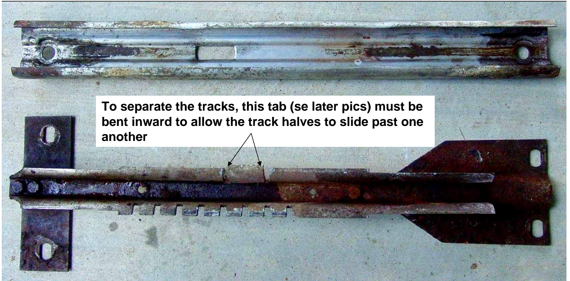
Upper (top) and lower seat tracks separated
