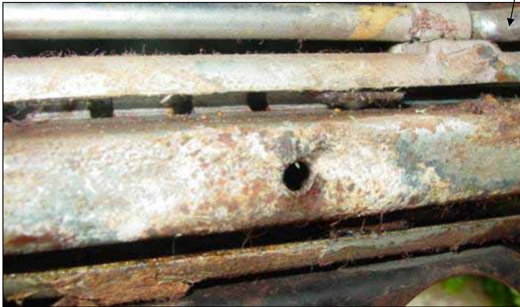
Underside of seat track with the adjuster release rod
