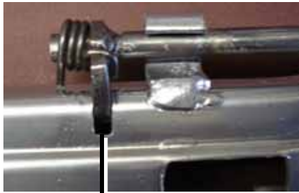
Seat adjuster rod engages in these slots
