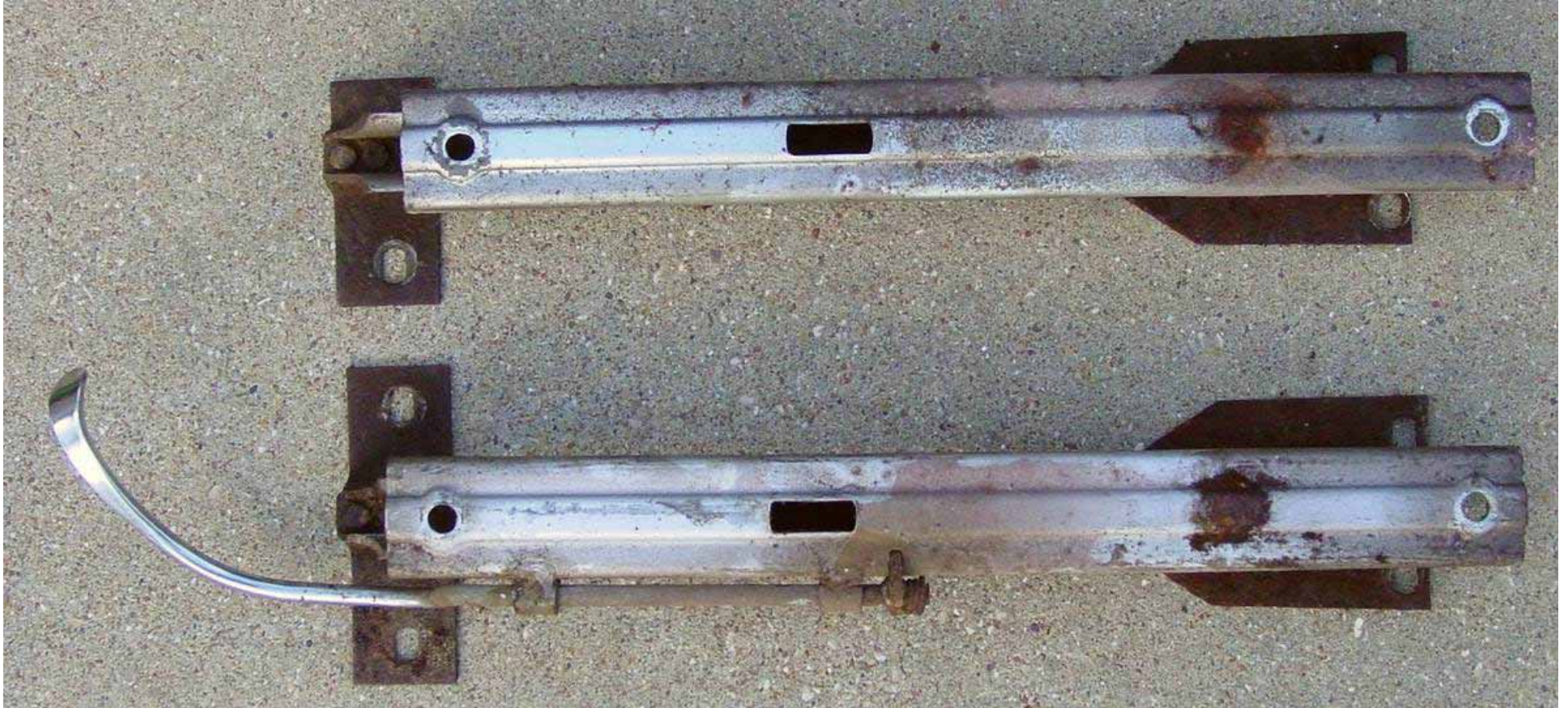
Seat tracks as found in the 1960 Lot's of rust!
