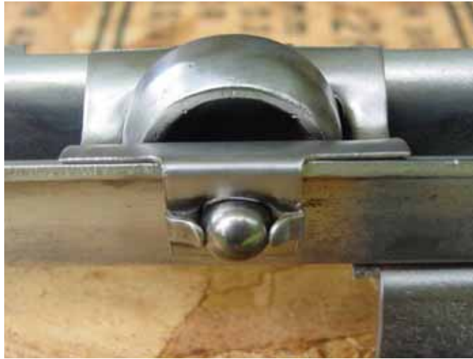
Seat track roller in bearing cage as it rides in lower track
