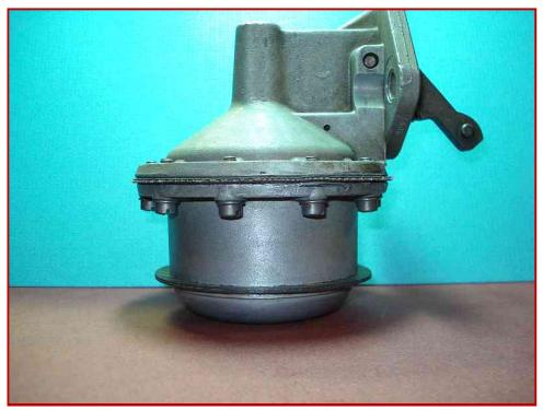
Note: replace the inlet and outlet fittings before you install the new pump.
