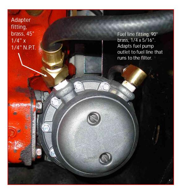
Fuel line fittings attached to the fuel pump body. The 1960 A.I.M. indicates that the 45° elbow should be rotated 15°-20° from vertical toward the right side.
