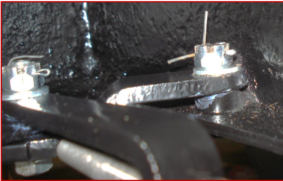
Lever mounts on stud welded to frame
