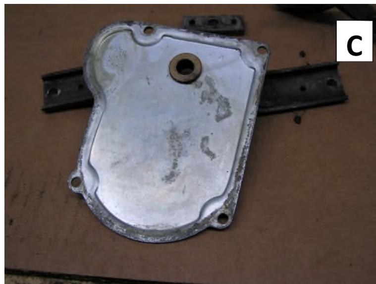
The end case cannot be plated unless the brush board is removed. If desired, simply drill out the 4 small rivets from the inside and lift the board out.
