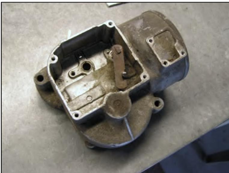
Now for removal of the drive cog from the rear case. Stake both the shaft and the cog (i.e., lightly punch or scratch the cog and shaft to make alignment reference points) to maintain proper alignment on reassembly (A). Drive the shaft from the cog using a drift. Remove the shaft and link assembly (B). The rear cover (C) can now be cleaned and prepared for plating along with the front cover.
