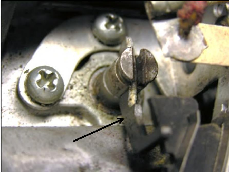
Remove the clip and washer from the park trip lever (oscillating arm), then using a pry tool, carefully lift the lever from the slotted shaft. This is what the parts look like after removal.
