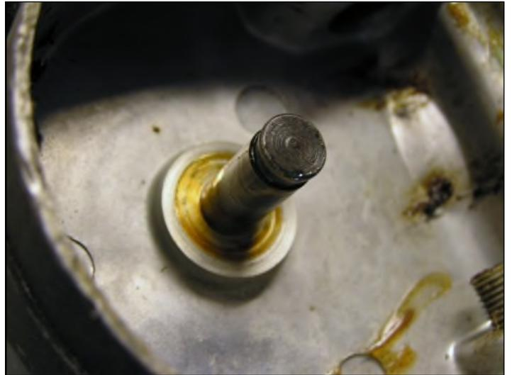
Now you can remove the armature from the housing from the commutator end (where the brushes make contact). There will be a bearing ball, felt donut, and spacer/disc located in the motor case bearing. Sometimes the ball will be stuck to the end of the armature.
