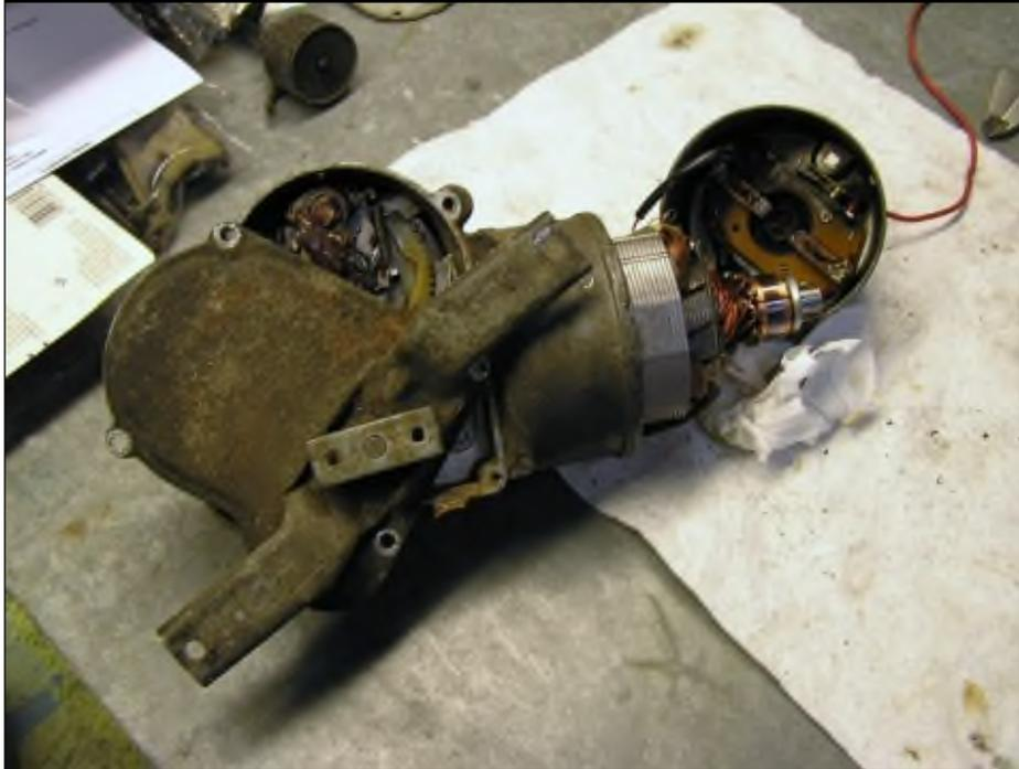
There will be an E-clip (**A**) holding the link lever to the gear mechanism. Remove the E-clip, and lift the link from the shaft. You can barely see it under the old red grease. Note there is a small spacer washer below the link lever. Also remove the spring (**B**) attached to the lever shaft, shown in the lower right of the photo below.
