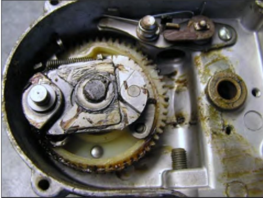
Remove the C-clip (**A**) and shim washers (**B**) from the shaft, and lift the gear out of the housing. Note there will also be a shim washer (**C**) below the gear.
