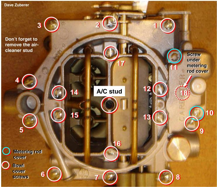
Here is a photo of a WCFB carb which should print at actual size of the carb. You can use it to make a template to make a "screw holder" useful when you disassemble the carb(s).
