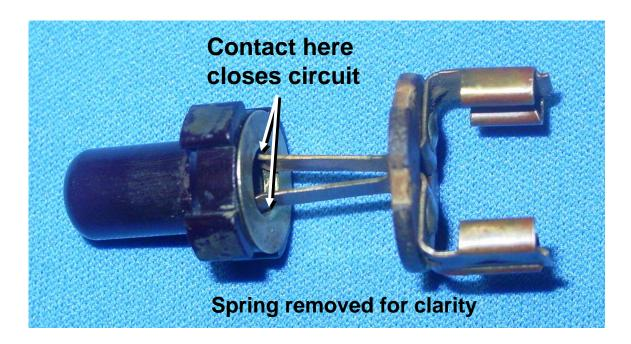
Door open, button is out: leads make contact with the brass ring to close the circuit and light the courtesy lamp.
