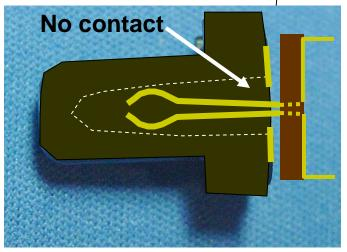
When the door is closed the button "squeezes" the contacts away from the brass contact on the end of the button and the circuit is open: lights out. When the door is open, the button moves forward allowing the contacts to expand and make contact with the brass ring on the button to complete the circuit: lights on!
