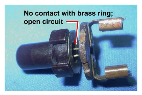
Door closed, button in: leads do not contact the brass ring so circuit is open
