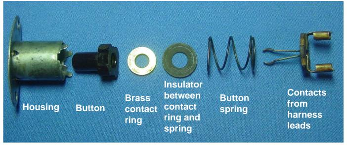
After rewiring our 60, the passenger door courtesy lamp switch was not lighting the lamp at all and the driver side was "jittery". Here is what I found when I opened it up. It's a fairly straight forward mechanism similar to the brake-light switch.
