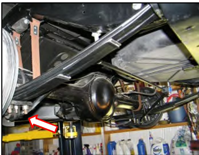
Lower shock mount plates and stabilizer bar brackets reinstalled on the spring/axle.
