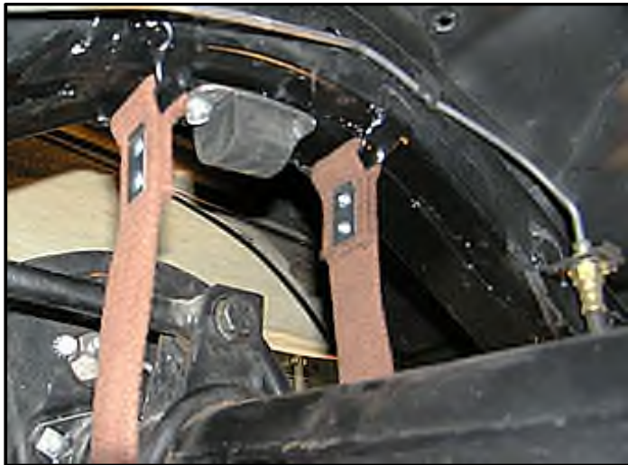
All four strap loops through the frame brackets and properly riveted.
