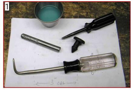
Push the rubber tip, while stretching the leg, into the tool until it's all the way in against the rubber cap (Fig. 3). It stretches 1 1/4" and stops inside the tool so it doesn't punch through the tip.
