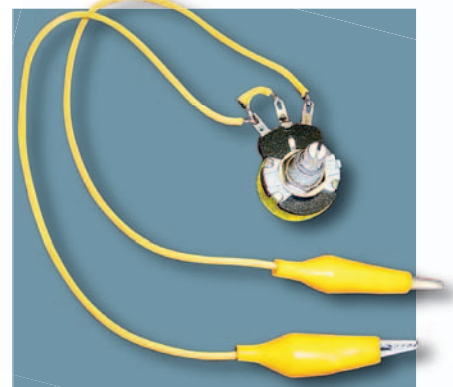
Here's the five-dollar diagnostic tool made from a Radio Shack 0-100 ohm volume control. It simulates the fuel sending unit to check the gauge and wiring.
