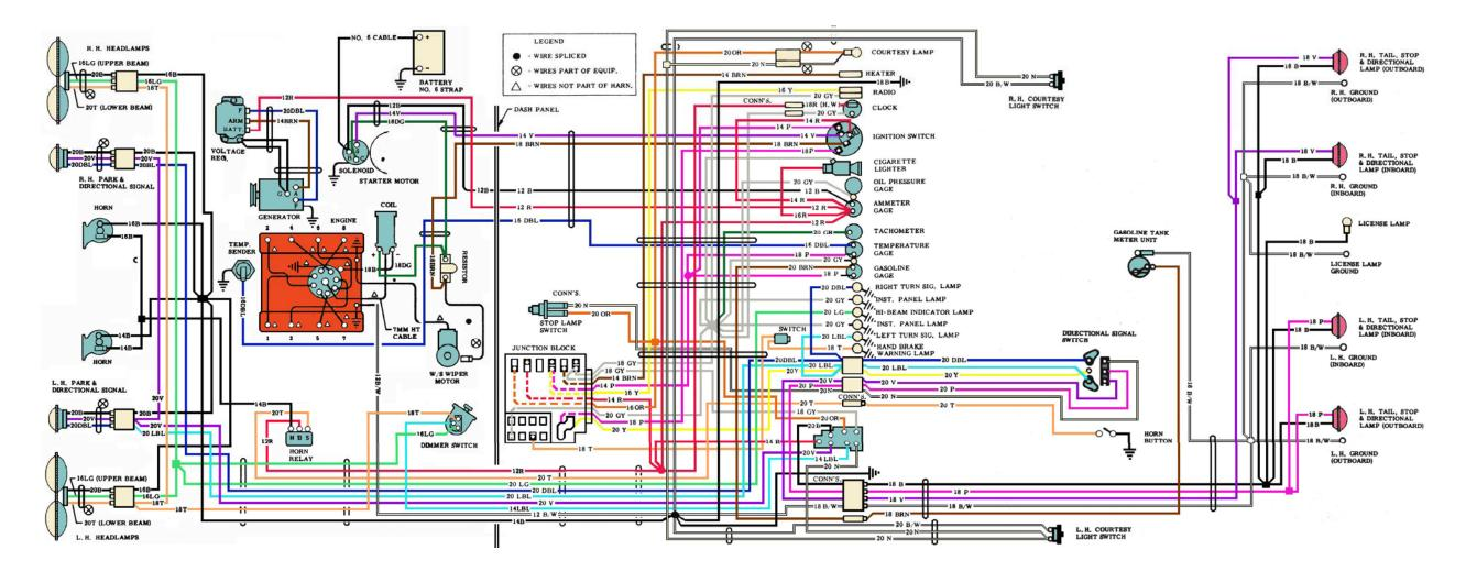
This drawing contains the ammeter wiring error – the leads coming to the rear of the ammeter need to be reversed. If it wired in as presented on this drawing the meter will show a discharge when charging.
