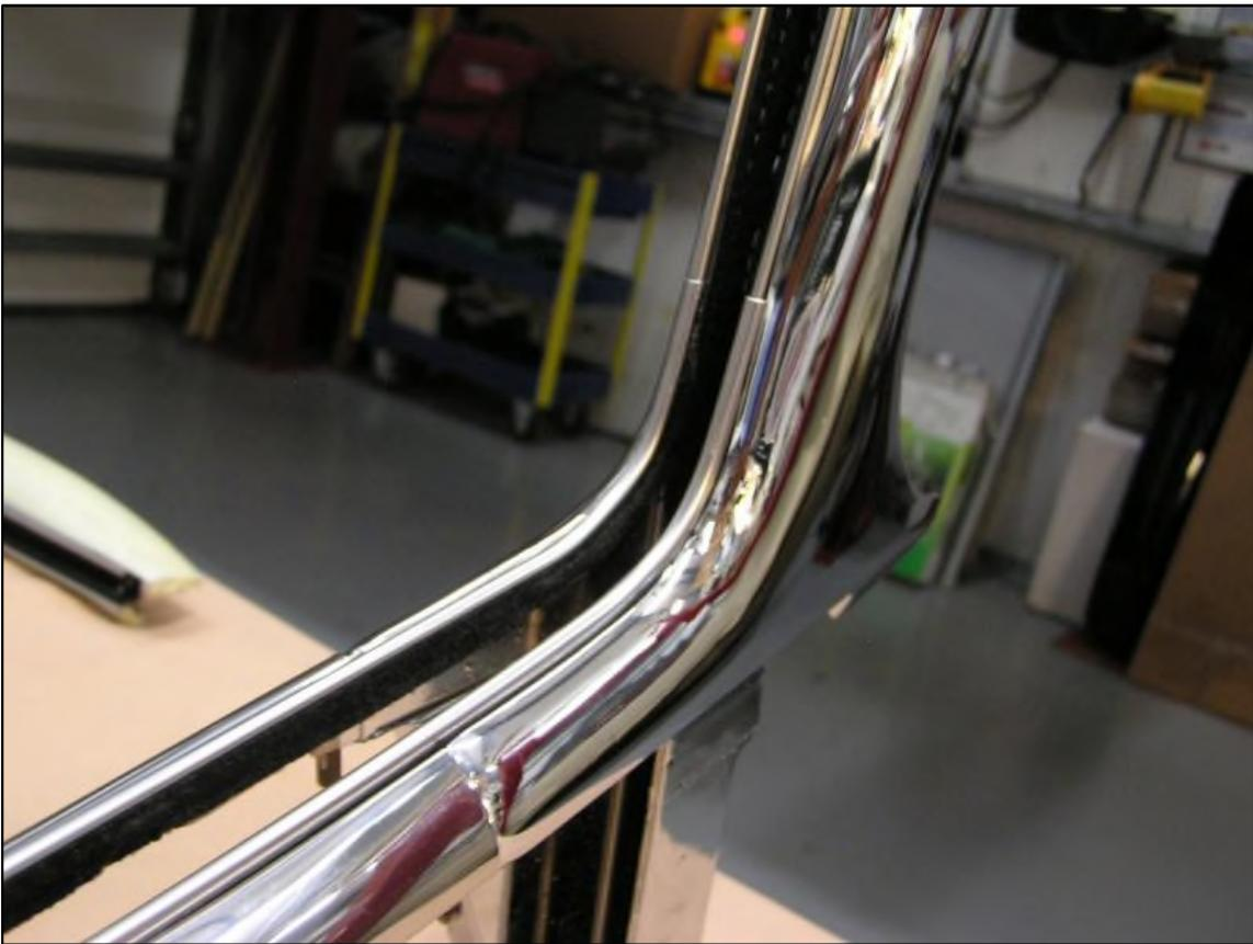
Here are some photos with the glass used for a test fit. The front frame of this window glides easily past the corners and fits well. Because I removed that thick area at each fuzzy corner there is no resistance to bind up the frame. At the rear end of the fuzzies, the frame may bind slightly.
