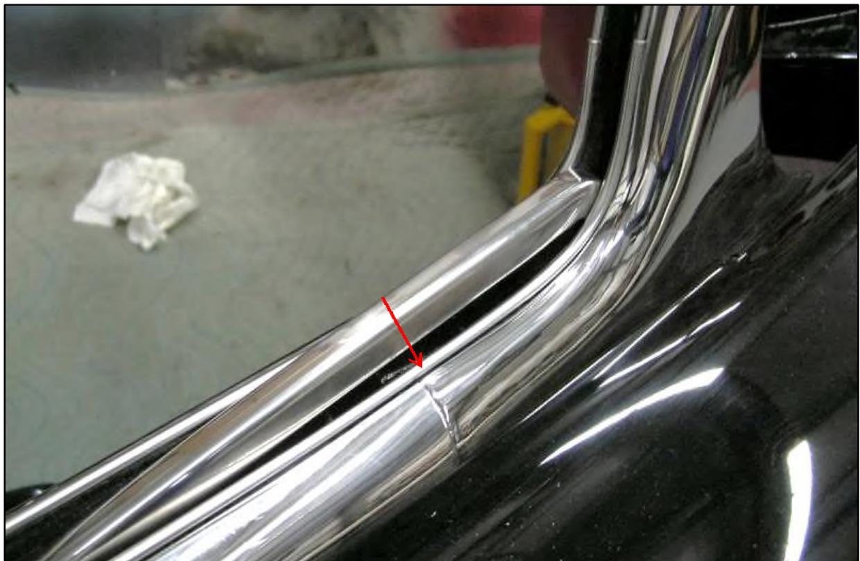
After the grinding for excess chrome removal, all 4 trim pieces now fit properly. You can see how much material needed to be removed.
