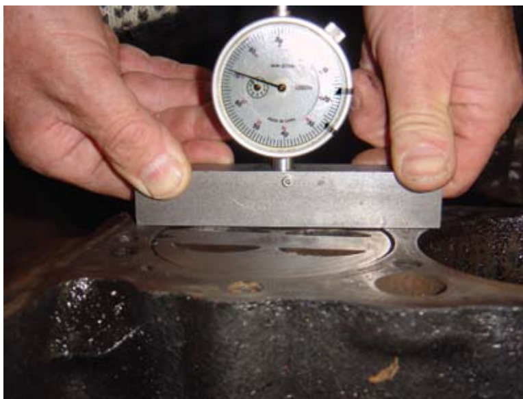
Setup for checking deck clearance. In this case the clearance of the original Flint-built engine is being checked prior to disassembling the block. It will be checked again during the assembly phase with the new KB157 pistons that have a specified compression height .003" greater than the OE pistons. All other things equal, the measured deck clearance of the newly assembled short block should be .003" less.
