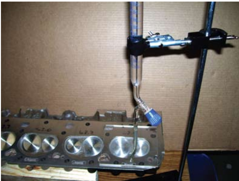
Homemade apparatus for checking head chamber volume. The equipment was purchased at a lab supply house, and the fluid is denatured alcohol with food coloring dye added.
