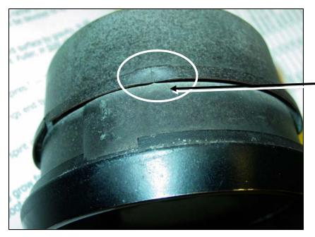
To separate the two halves of the clock housing, gently pry up the crimped spots as shown at left.
