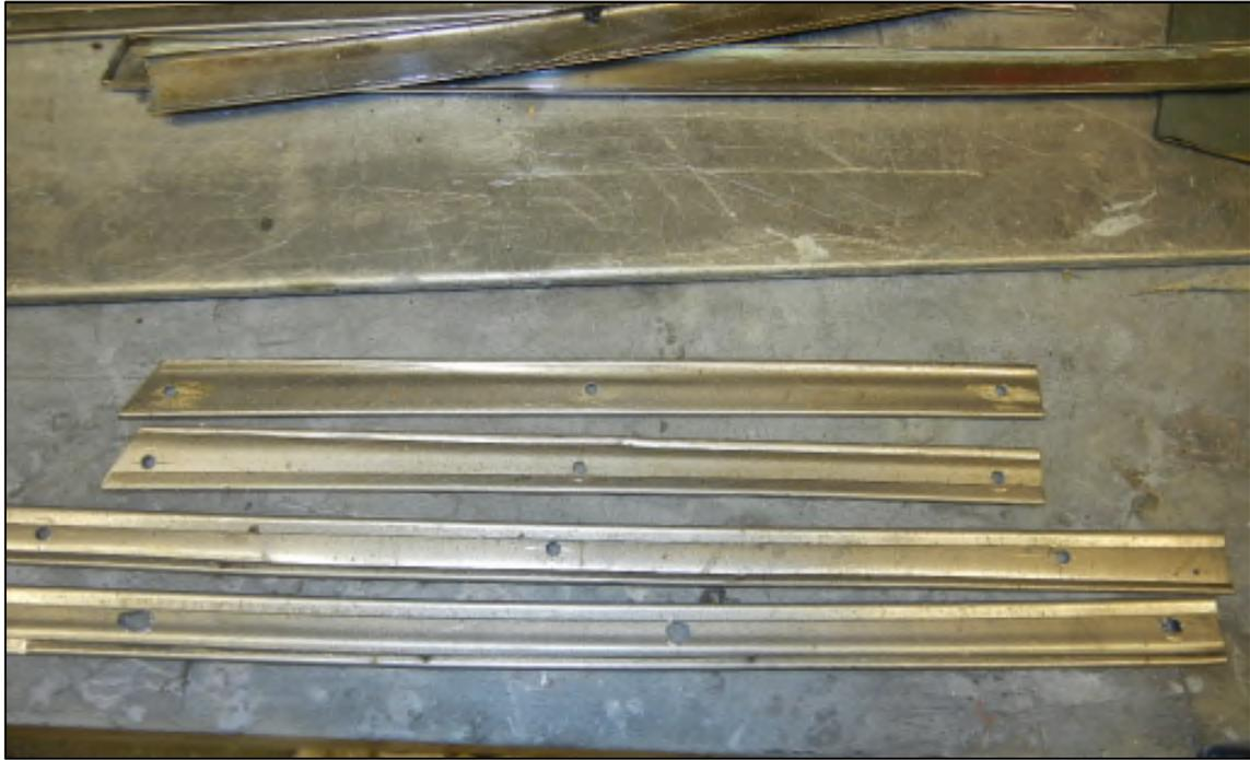
Before installing the T-Bolts and putting stainless on the retainers, I put some strip calk on the bolt to hold it in place
