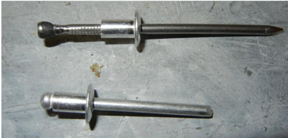
I put some strip calk on the end of the finishing nail to hold the rivet in place while I stuck it in the hole and this also helped hold on the washer and also filled up the hole to prevent leaking.
