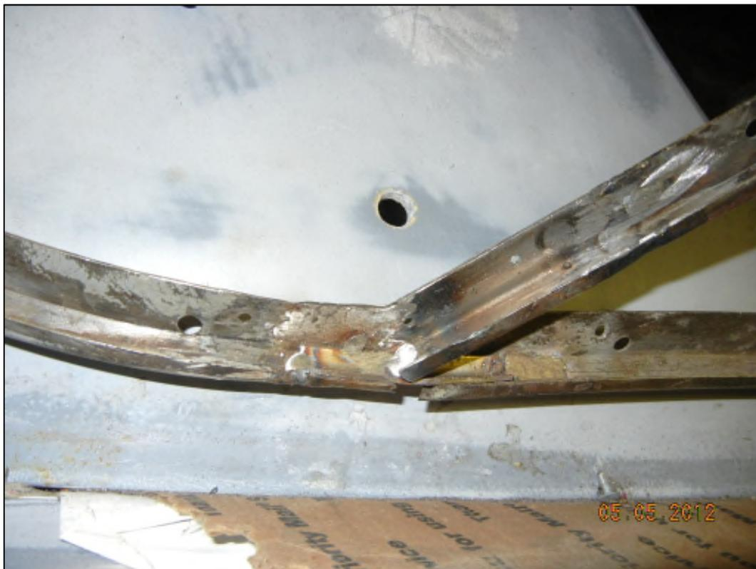
After repairing the frame and any of the stainless you work on, you need to remove all the glue, cement, sealer and crap from it... this ESPECIALLY includes all the lips on the stainless moldings. I flattened out a nail and bent it over at 90 degrees and used this to go inside all the trim grooves.
