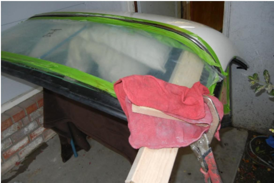
7. Before cutting the holes in the rubber, make sure you have the window in the right place! What I did was to sharpen a nail (as I didn't have an ice pick) and using some WD40 spray the nail or ice pick and stuck it through the hole. Glassworks makes a "barrel" drill that can go over the nail and drills a hole...pretty handy, but as far as cutting a nice clean hole....that didn't happen. Once I had the hole drilled, I went back over them with a drill bit to clean them out.
