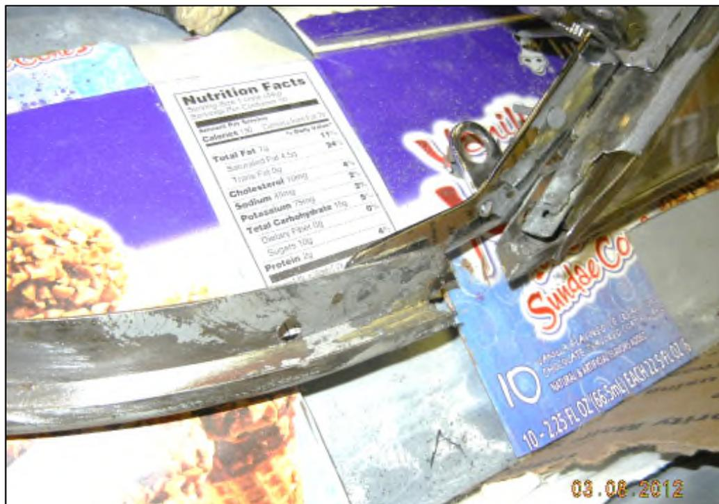
I then got some stainless and bent up a section and welded it back in place using the bracket as a guide.
