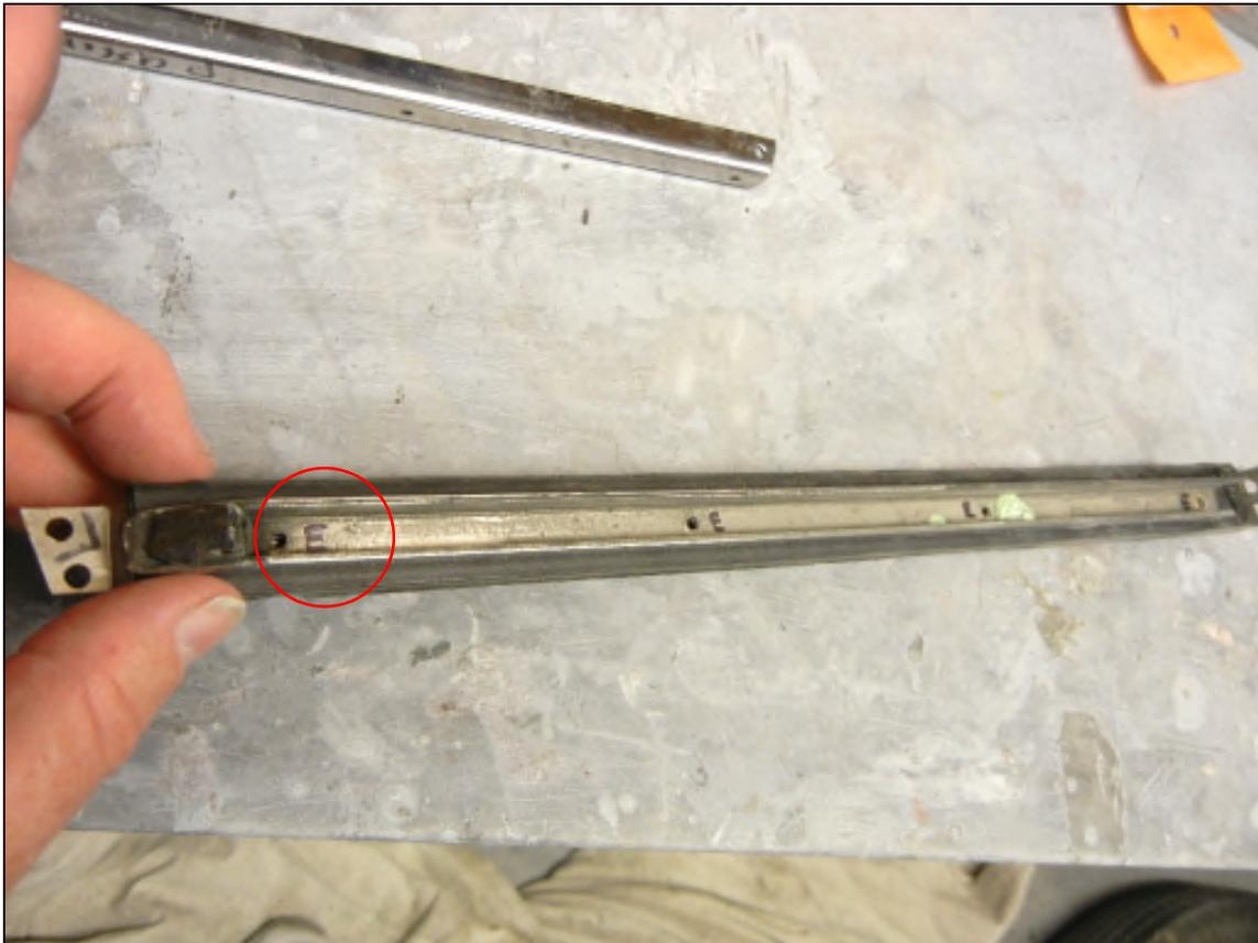
Stainless molding retainers that a friend of mine at a machine shop made out of galvanized steel. You cannot buy these. The reproductions are made out of plastic. Plastic?? No thanks! They say they work and they don't rust, but personally I question the durability and strength. Should you wish to make your own, note that they have a slight curve to them and also check the spacing so the T-Bolts will fit.
