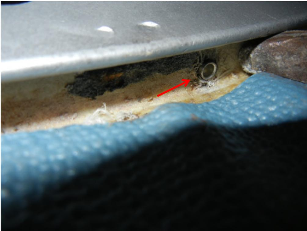
I thought about using screws, but trying to get nut drivers on the inside of the frame was almost impossible. I decided to use pop rivets. Some may joke about pop rivets, but I can assure you that your fiberglass will tear before a pop rivet does!
