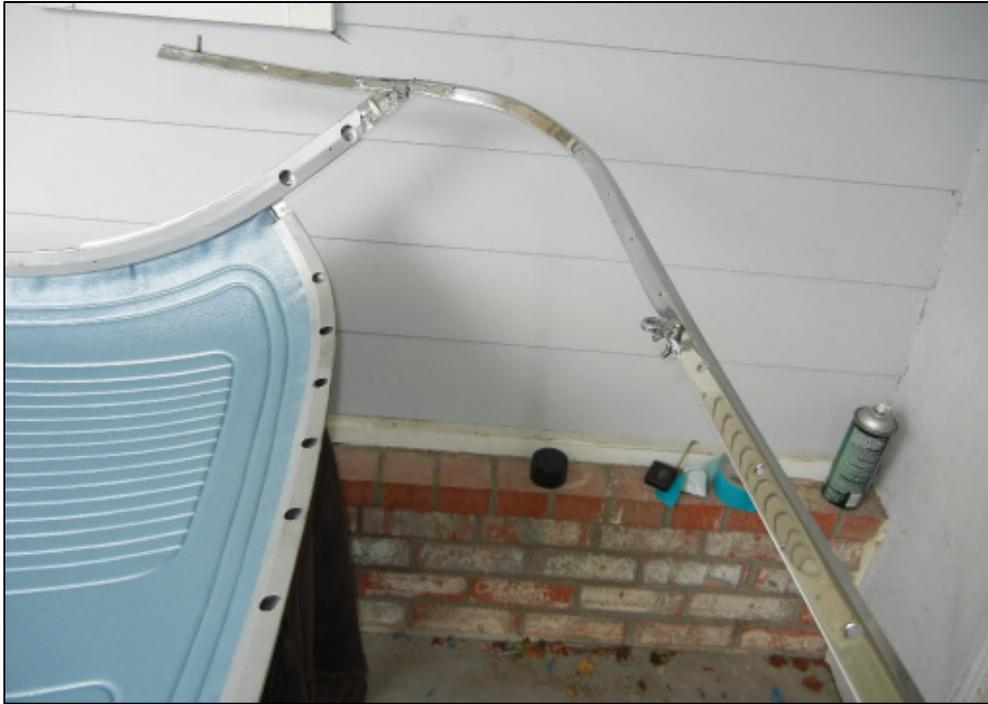
Since my hardtop bracket was cracked...forget repairing it! Any repair you do will probably not hold up as the bracket is made from brass. Some think it's pot metal but mine was solid brass.
