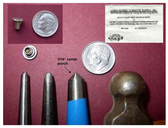
Peening the hinge pivot rivet:
