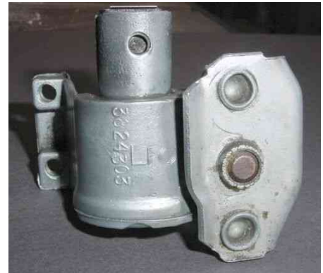
Regulator showing the normal “peened” pot- metal studs holding the backing plate.
