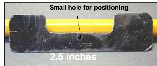
“Butterfly” reinforcement for door-panel clip holes.
