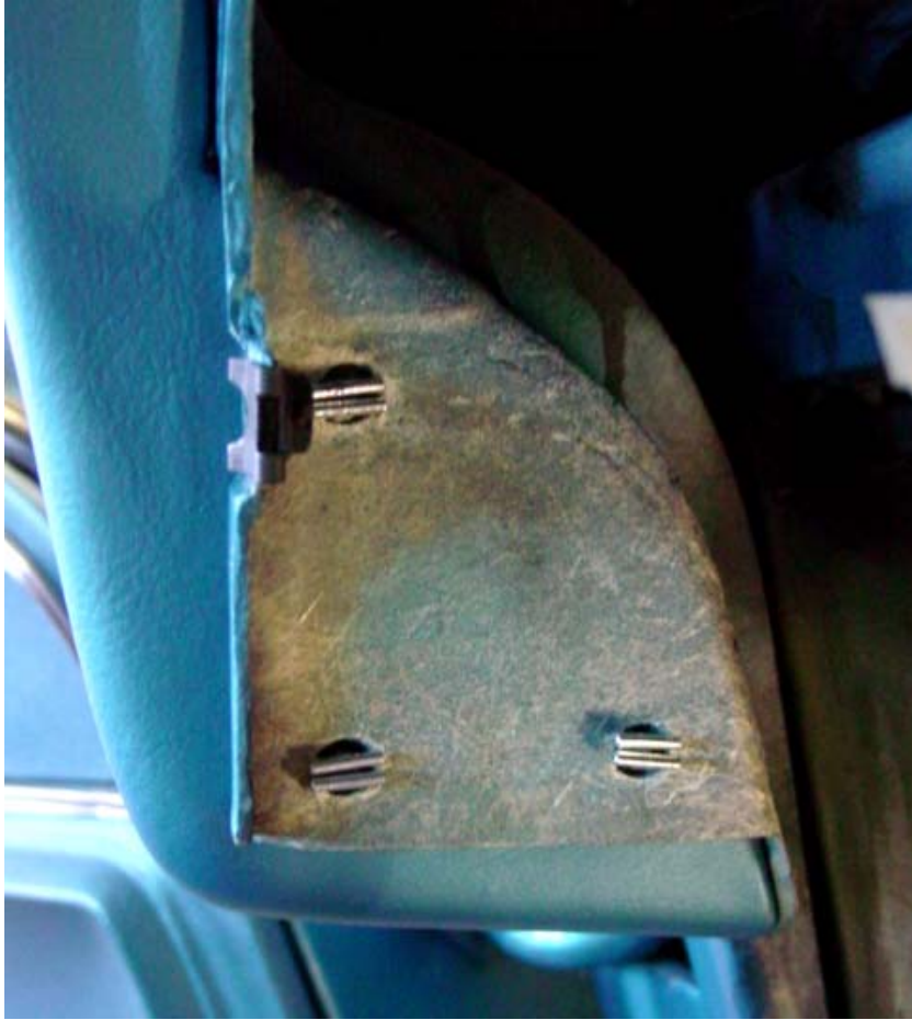
Clips installed in outboard side of the dash pad surrounding the instrument cluster
