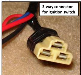
Locate the Brown wire terminal space. Using a small flat pick tool or screwdriver, insert its end into the open front portion of the plug. Push in to flatten the small tab of the terminal to allow it to be removed from the wire side. Remove it from the plug.
