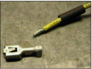
Precut and install some heat-shrink tubing onto the wire, **away from heat**. Solder the terminal to the wire and install the heat shrink. A butane lighter is convenient for heating the heat-shrink insulation.
