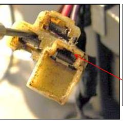
Slide thin blade in these slots to depress the locking tab on the connector. Pulling gently on the wire while you insert the blade will usually release the connector from the plug. You can see the tabs in the connector at left.
