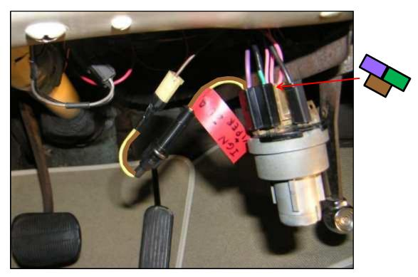
Reinstall the switch to the dash, ensure a fuse is installed and test the electrical system.
