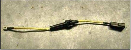
At the ignition switch plug, bend the lock tab of the fuse-holder female terminal slightly and install into the 3-place plug where the Brown wire terminal was originally located. **Rewrap the harness tape back around the plug**. Use electrical tape to get a good tight fit if needed. Plug the other end of the fuse-holder connector to the Brown-wire terminal that you made up.
