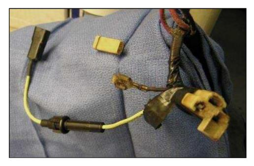
This modification is one that **will protect just the ignition circuit**. But keep in mind that if a poor connection or fault occurs in the wiring, the engine will shut down. Be aware that this could happen. But like any motor vehicle, any failure in the ignition can shut the vehicle down. We see this happen on modern cars as well, and are aware of recalls even in today's high-tech world. Mistakes happen.
