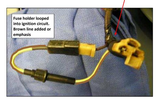
Reinstall the plug to the back of the ignition switch. Ensure the fuse is installed, reconnect the battery; check all circuits for proper operation. Start the car to ensure your wiring is correct. As a test, run the engine and wiper motor simultaneously to verify its function and the fuse is an adequate rating. You can place paper towels or cloths under the wiper blades to prevent scratches to the glass when running the wipers.
