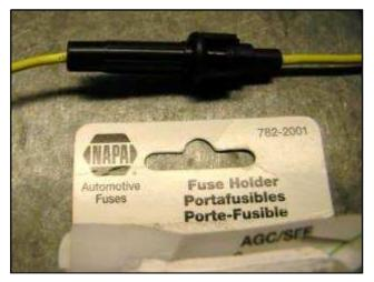
Acquire a **female terminal** from your old harness or get one at an Auto Parts store. It must be the locking tab (Packard Series 56) type. You can salvage your old terminals by spreading the brass collars, cleaning out the old wire and soldering the new wire to it.
