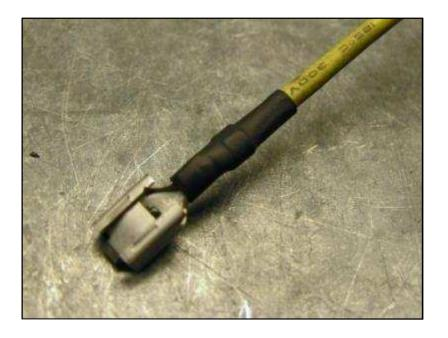
On the opposite end, Prepare a **male terminal** blade with heat shrink. If you have old harness connectors, locate a male terminal (lock tab type) with plastic insulator plug as shown below. This type is actually used on the 1963 up GM cars and Corvettes.
