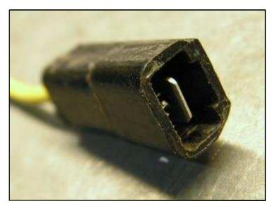
Here is the completed "plug-in-ready" fuse holder.
