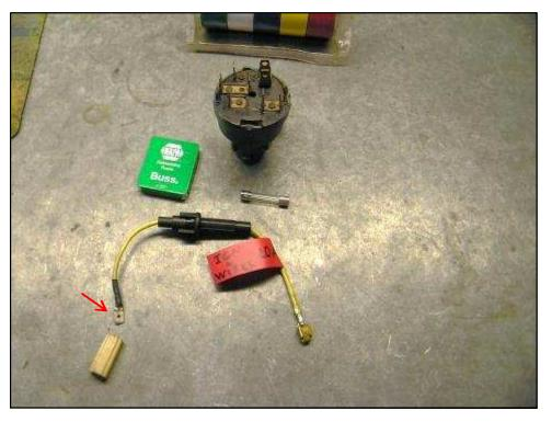
Below is the '56/'57 Ignition switch. The fuse splices in to the IGN-1 terminal which is the **Brown wire**.
