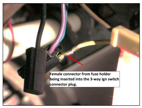
Connect the male terminal end of the fuse holder into the female connector on the Brown wire. Tape up the connection for safety. Connect the remaining wires to the switch.
