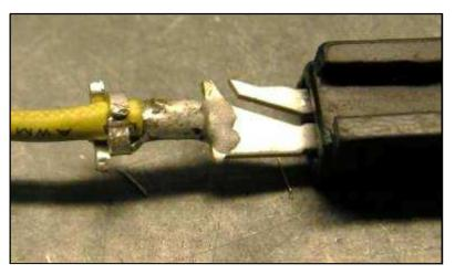
Install your chosen male terminal to the wire by soldering. Here I've used the GM type.
