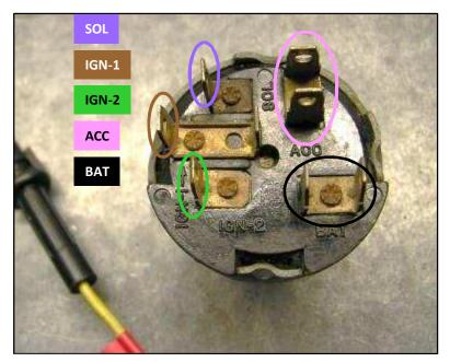
The **Purple** wire is the **Solenoid** input at the Starter. The **Black** is the **Main Feed +12V** from the Ammeter. The **Green** is the **coil +** direct feed described above. The 2 **Pink** connectors are the **ACC** (Accessory) feeds to the Auxiliary Fuse Panel for the Turn Signal flasher, Gauge power feeds, and the radio and heater if so equipped.
