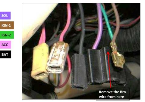
Insert the brown wire female terminal into your plastic connector after bending the lock tab back up a bit.
