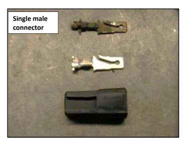
If not, just use a male blade type and plan to tape the connection later.
