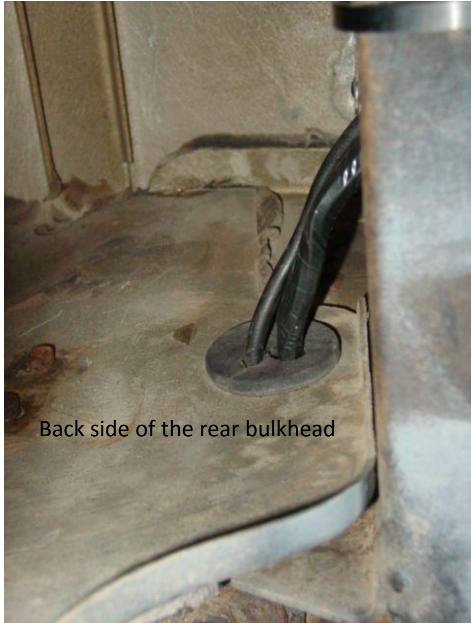
Cable connection to repro power antenna. Difficult to get to if you have under-car exhausts. Mufflers are in the way.
