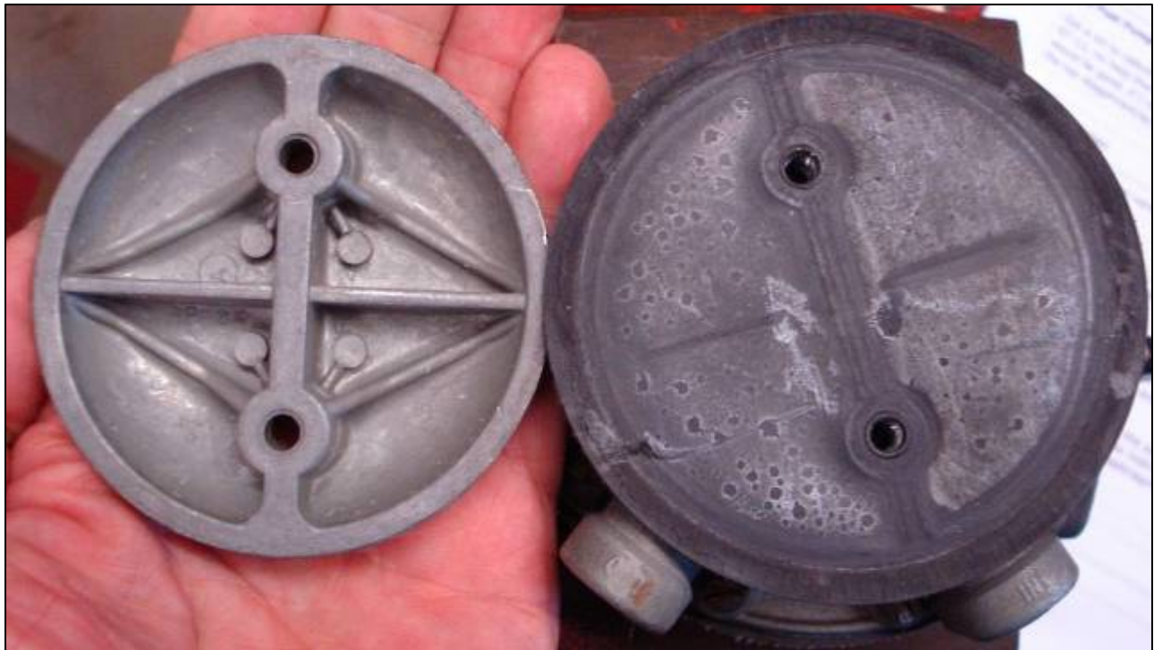
Pulsator cover removed to reveal pulsator diaphragm
