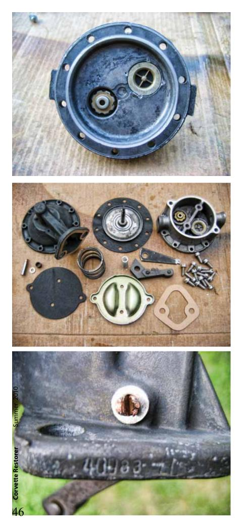
Re-use original link, main spring, and rocker arm along with new bushing and rebuilt diaphragm/stem assembly as shown in Fig. 20. Apply moly grease or chassis grease to all sliding surfaces, fit hook of link into slot of stem with open end of hook facing up. Insert bushing onto link/rocker arm articulation point. Use the same pulling/twisting procedure used for disassembly. This may require you to go back into the house, kick the dog again, and have a coupla more brewskis.
