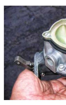
moved it. Place the X marked end onto an anvil or vise, and, using a small cold chisel and light hammer, gently deform the pin by re-spreading the same grooves that you squeezed together upon disassembly (fig. 21). Insert small return spring between rocker arm and upper casting (fig. 22).
