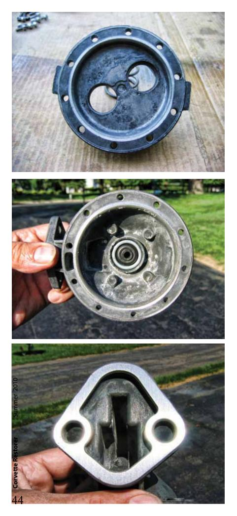
vent. Be sure to clear the two diaphragm vent holes in the upper section with a small drill bit or needle file. Use a toothbrush to remove heavy deposits. Blow dry with compressed air. There were two types of pulsator covers used for this model pump—the cast pot metal and a cadmium-plated/dichromatewashed stamped steel. The stamped steel type requires washing, surfacing and finally either plating or painting with artificial caddichromate finishes.
