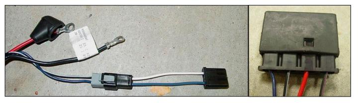
The photos shown here were taken when we rewired our '65 A/C coupe and swapped out the alternator for a 12SI (3-wire, internally regulated) model. The harnesses were obtained from Lectric Limited along with their conversion harness for the alternator change.
