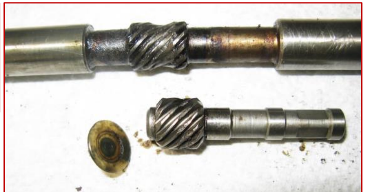
Tach-drive cross gear and shaft badly damaged.
