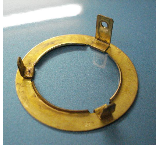
“Lower” horn contact in turn signal switch. Tabs slide into slots in the switch housing.
