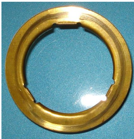
“Lower” horn contact in turn signal switch. Tabs slide into slots in the switch housing.
