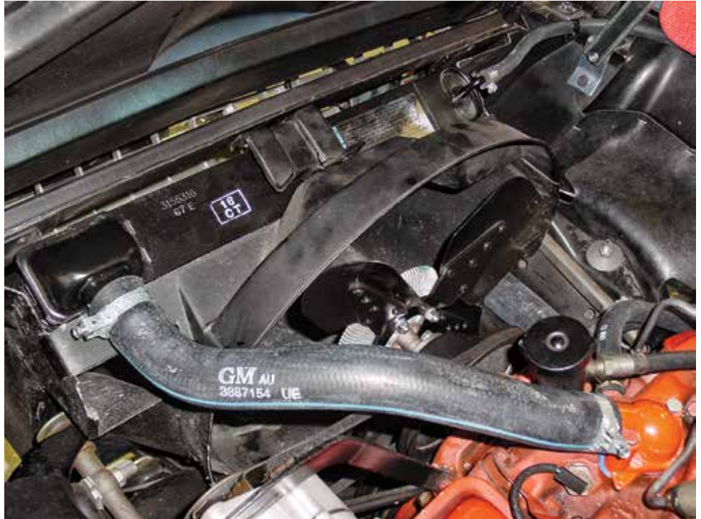
An overview of the complete cooling system on Corvettes
