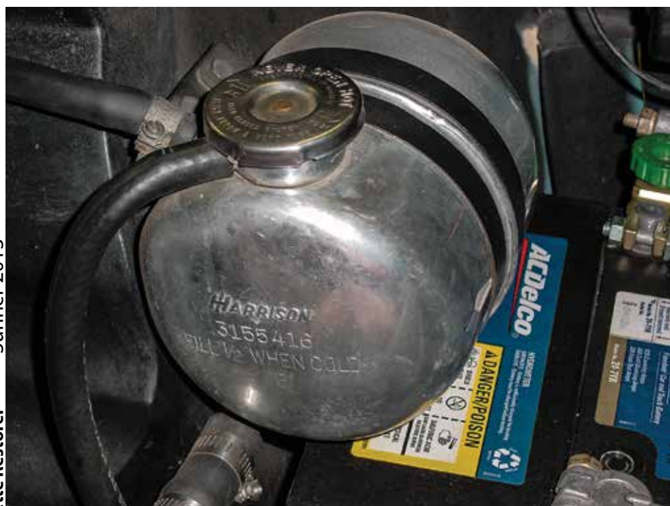
The Harrison aluminum expansion tank with the inlet and overflow at the top and the outlet at the bottom. Only fill half full when cold or it may puke coolant out the overflow during hot-soak.
