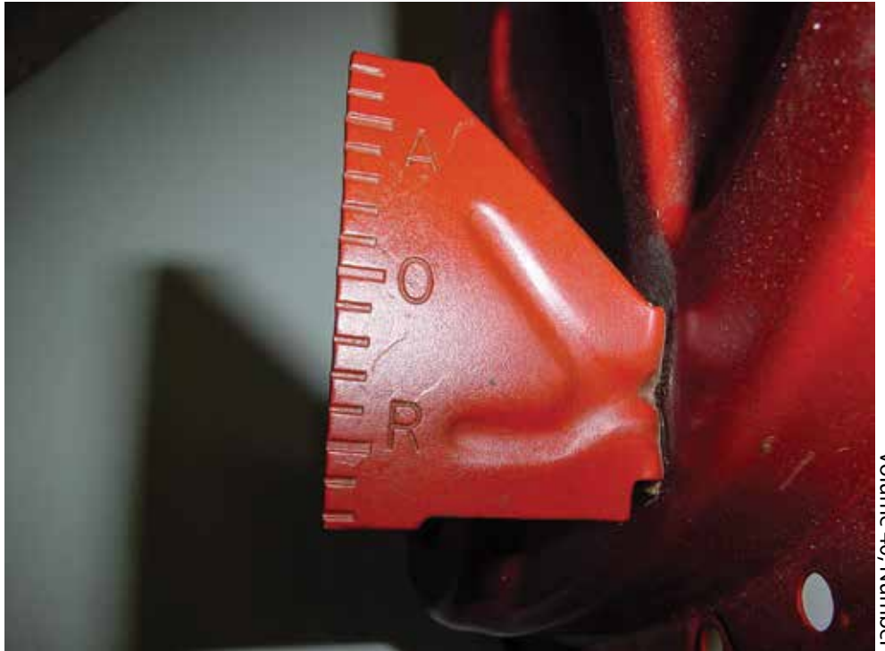
Setting correct initial timing and ensuring that vacuum advance unit is fully deployed at idle are essential for maximum idle and low-speed cooling performance.
