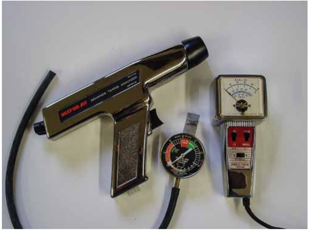
Basic tune-up tools are essential to set dwell, set and map timing and advance curve, and adjust idle mixture.
