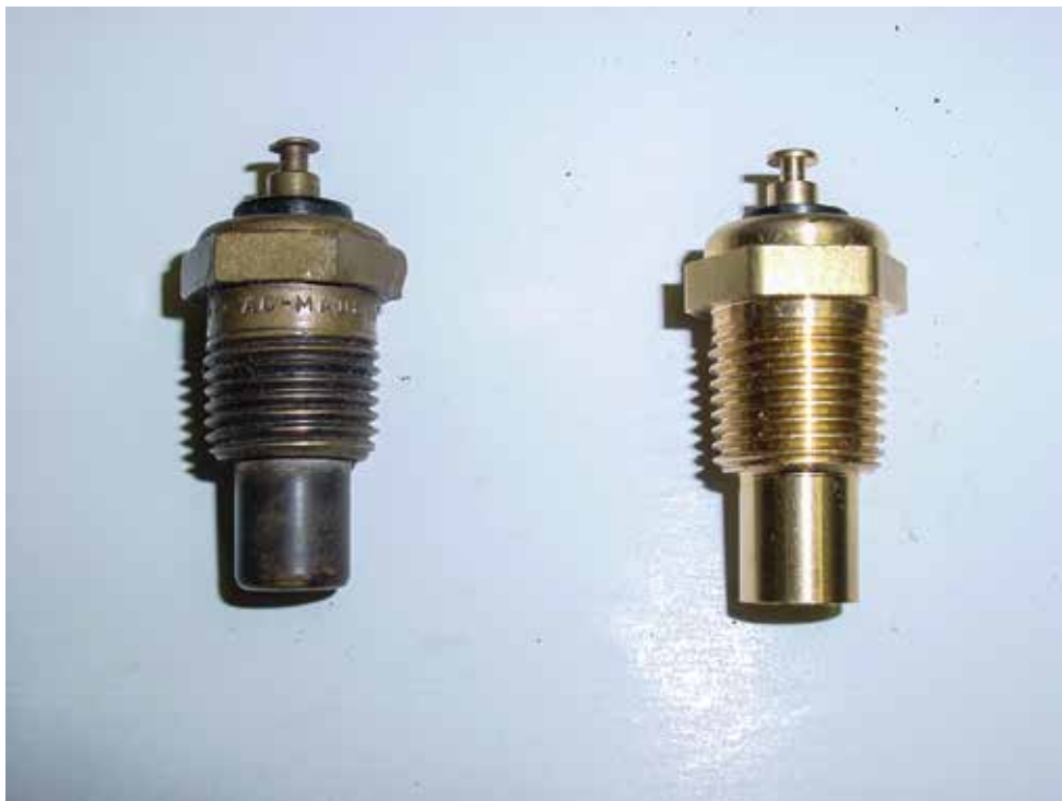
The original AC temp sending unit on the left, and a Wells TU-5 replacement on the right; calibration of replacements is always suspect; check the gauge reading against an I.R. gun shot of the upper radiator hose.
