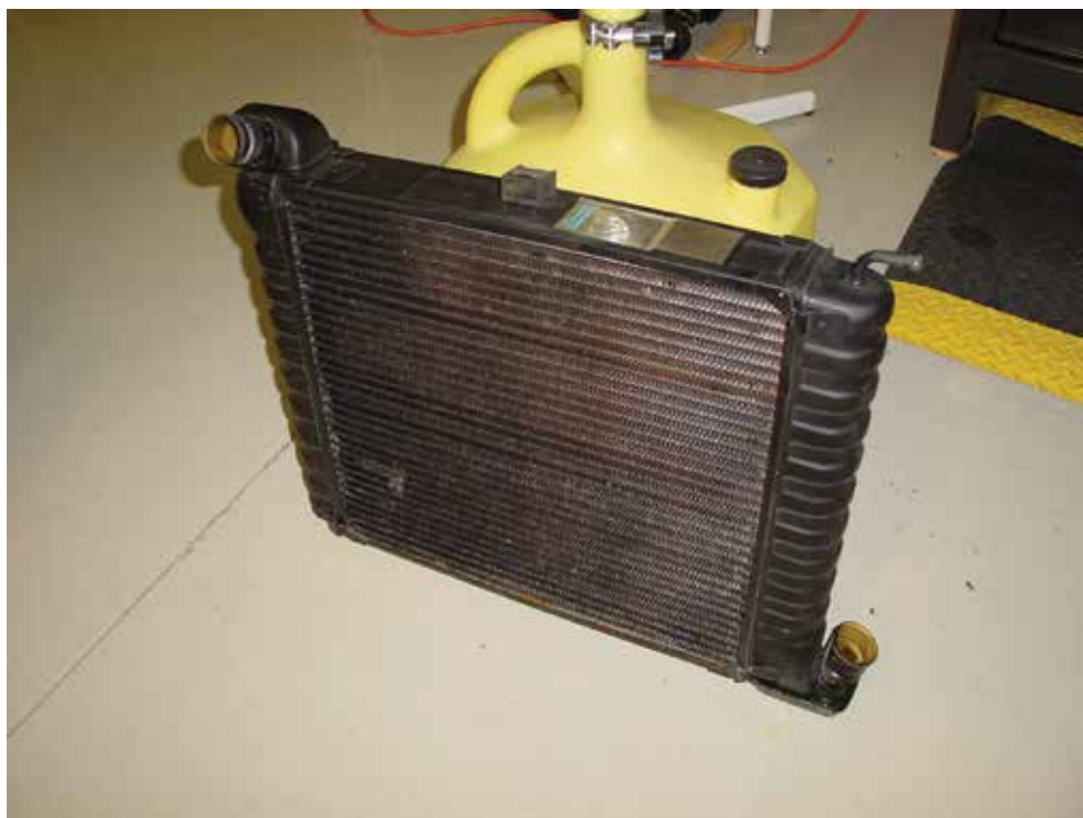
A typical look-alike copper/brass replacement radiator; note the rounded/stamped end tanks. These have about 30% less cooling capacity than the original Harrison aluminum radiator.
