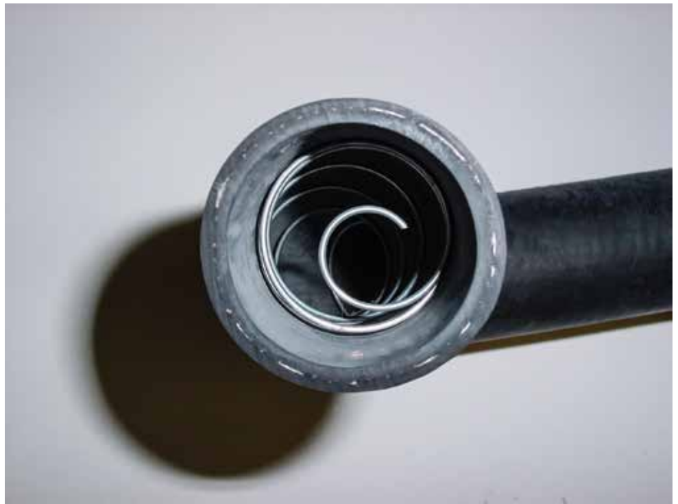
Original lower radiator hoses had this coiled steel wire reinforcement to prevent collapse. Modern hoses are made from better materials and generally don't need it.
