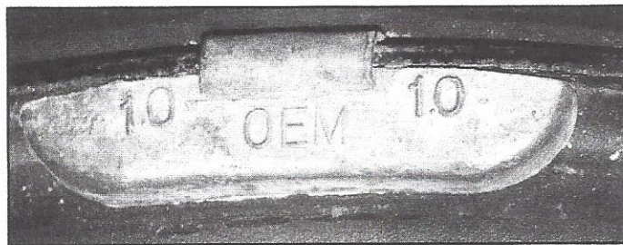
Fig. 7 – a one-ounce weight with the OEM embossing found on an original unused Goldline spare tire on a '66 Corvette, manufacturer unknown – photo courtesy of Peter Martin
