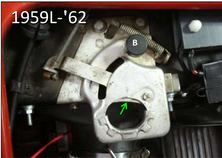
Both latches (top views) shown here in the “open” position. Note the retracted blade catches.
