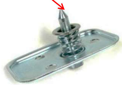
Late '58 to early '59 male hood latch. Note the slender pin like the '53-'57 but no provision for the bumper
