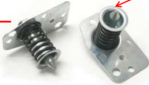
On the '53-'57 cars the adjusting "bumper" is attached to the male latch assembly.
