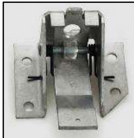
The female latches for the '53-'57 Corvettes were all the same. Note that the right-side latch has a tab/arm facing outboard for attachment of the cable while the left-side latch does not. The cables exit the firewall behind the latches (insets), pass through the hole in the lock lever and are anchored with brass barrel cable stops. Photos courtesy of Rich Mozzetta.
